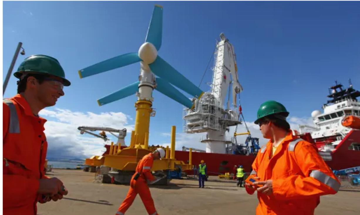
A tidal energy turbine is loaded onto a barge, heading for an Atlantis Resources test site off Orkney. Photograph: Jeff J Mitchell/Getty Images
