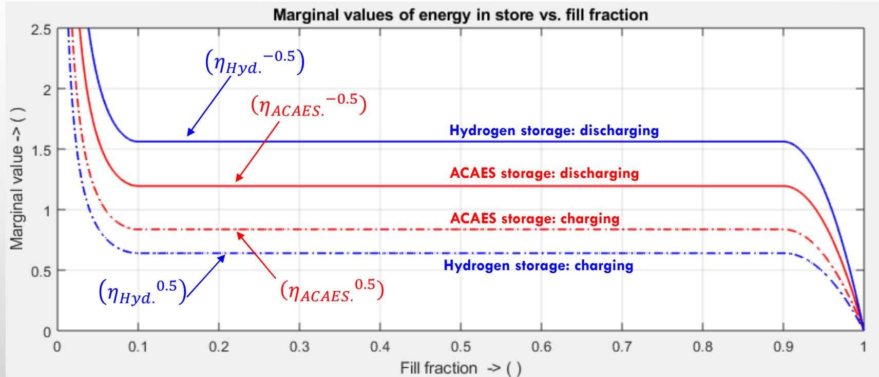
Within constraints, energy is preferentially put into the stores with highest marginal value and energy is preferentially withdrawn from stores with lowest marginal value.
