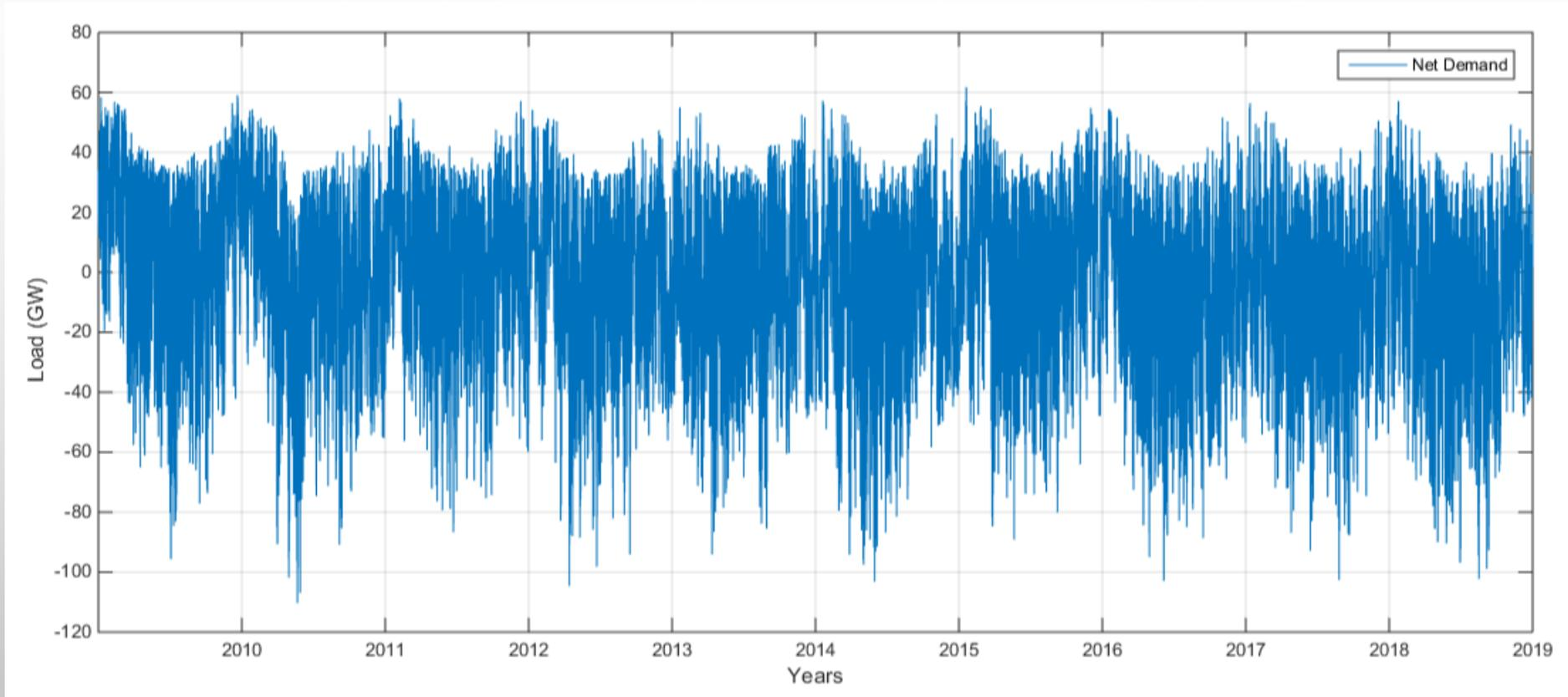
*Net Demand for the UK (2009-2019) with 75% of generation from wind, 25% generation from PV and 10% over-capacity (i.e. the average value of Net Demand here is slightly negative).*
