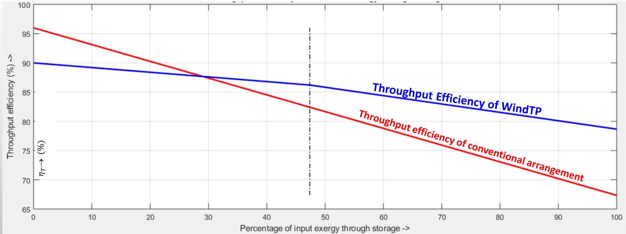
WIS works well when a high fraction of all energy from the wind turbines passes through storage.
