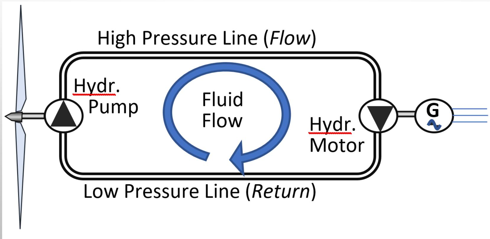
Note: hydraulic transmissions are the natural design choice for *Torque Machines!*
