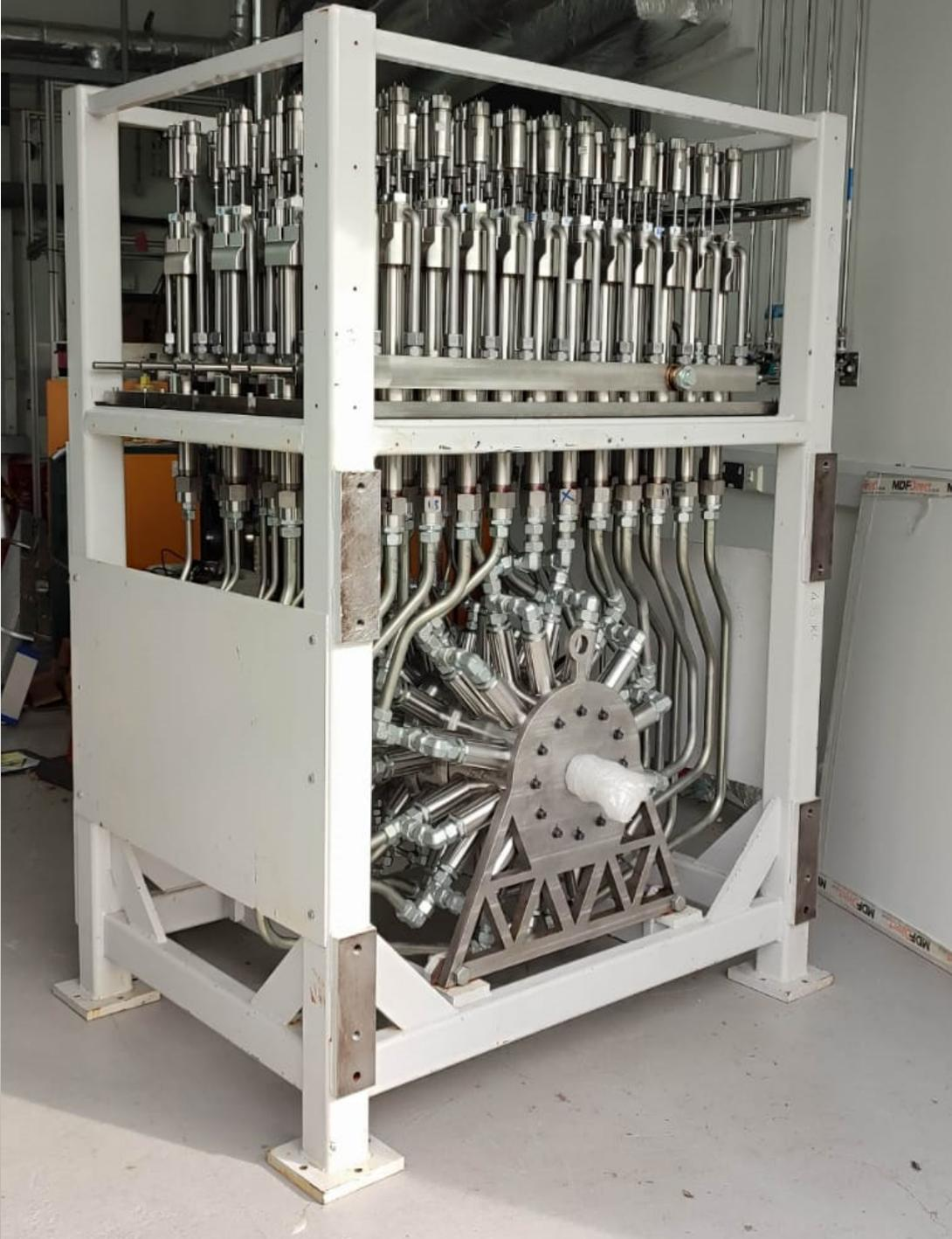
The machine consists of two parts. The lower half is the displacer, and the upper half is the converter. We have oil in the lower half to move backward and forward within pipes and this oil compresses the air in the converter pipes.
